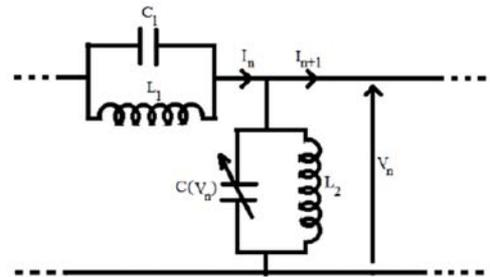
Figure 1. Model for the unit - cell circuit.
